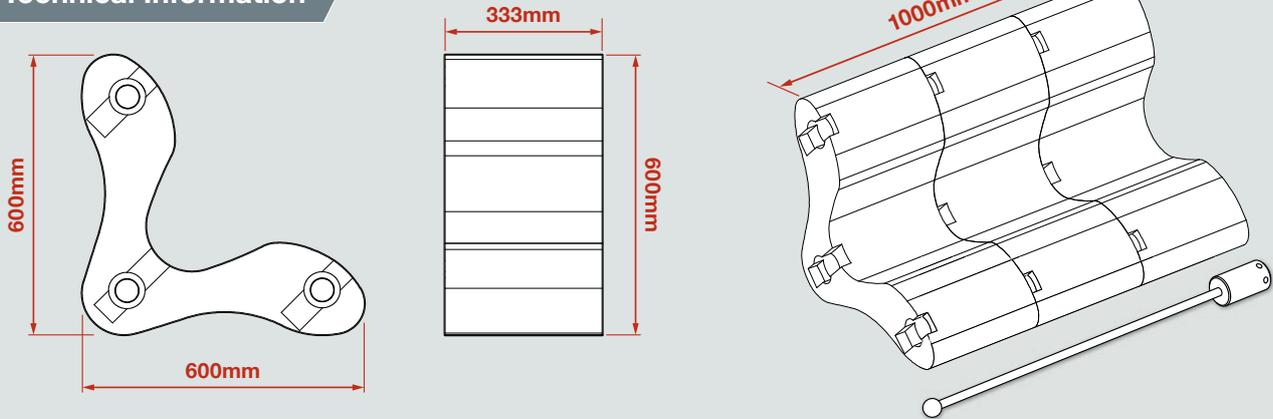
Manufactured from 100% recycled rubber and polyurethane, the Rapid Defender is supplied complete with steel securing rods and fixings.
